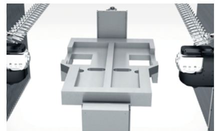
The A-axis enables free positioning of the workpiece.
